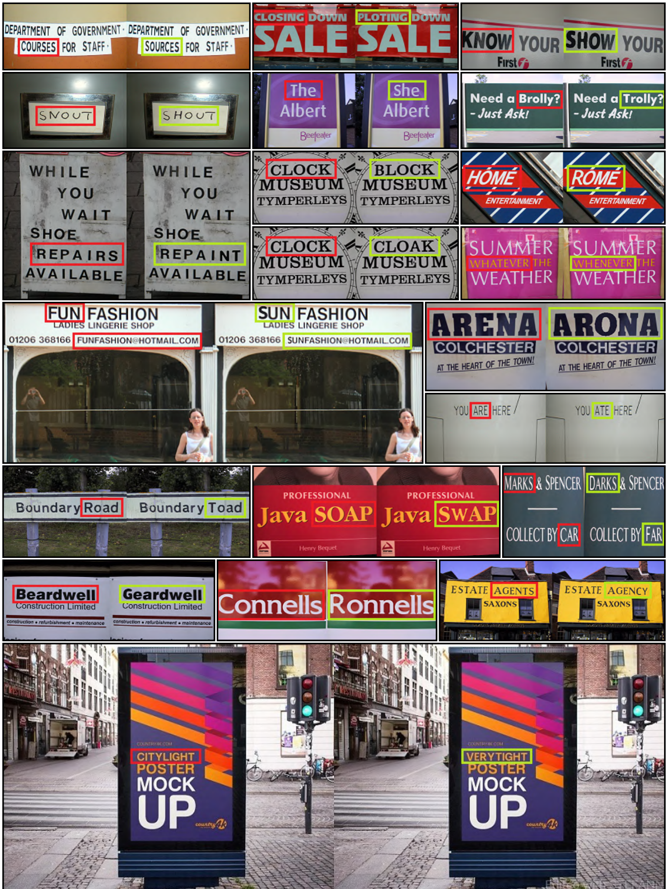
Figure 4. Editing texts in scene images with STEFANN. Left: Original images with text regions marked in red. Right: Edited images with text regions marked in green.
